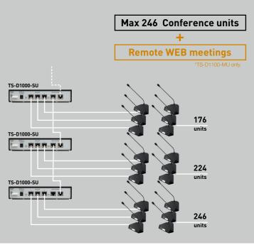
Function setting : Number of open microphones, Auto mic-off function, Microphone priority selector
